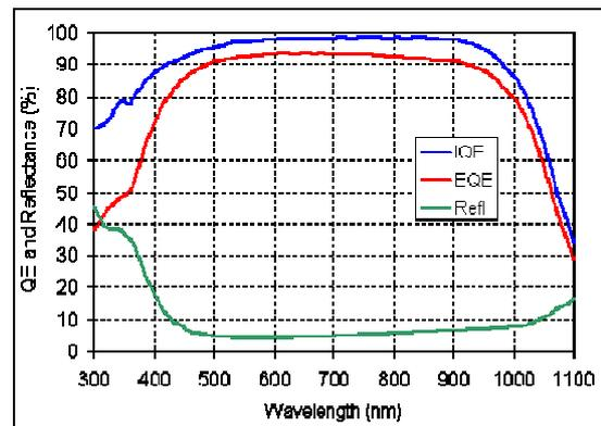
**Figure 4** QE and reflectance measurements of a characteristic cell made using the “Blue” Process. The excellent blue and red response indicates excellent surface passivation as well as good bulk lifetimes with implanted emitters.
