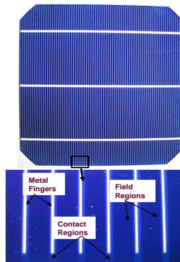
**Figure 4.** Optical camera image of a finished selective emitter cell showing the contrast in the differentially doped regions of the cell
