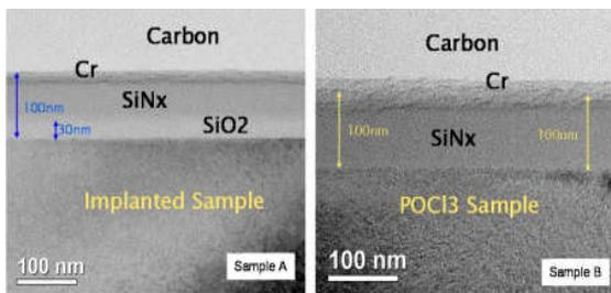
**Figure 2.** Cross-section TEM comparisons between Implanted and  $POCl_3$  emitters illustrating no residual defects in the crystal lattice in the implanted emitter. A smooth Si-SiO<sub>2</sub> interface and the presence of a thin passivating oxide are also evident from the picture.
