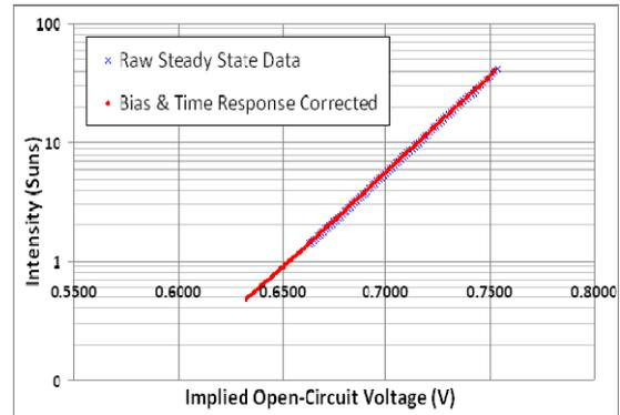
**Figure 3.** Implied Voc measurements on a 60ohm/sq implanted emitter indicating excellent surface passivation of the emitter and good bulk lifetime obtained after the activation anneal.
