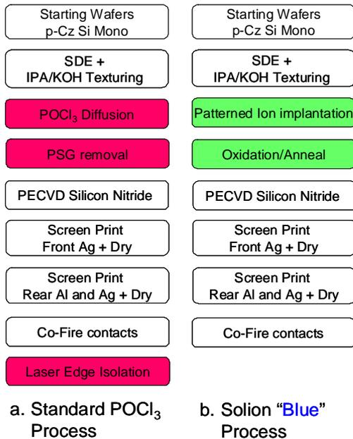
**Figure 1.** Process simplification for fabrication of Selective emitter cells using ion implantation. The Solion "Blue" process simplifies processing by eliminating complex diffusion recipes, the PSG removal wet etch step as well as the junction isolation step.
