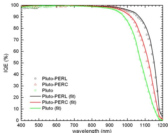
**Figure 3.** Internal quantum efficiency (IQE) curves of the best Pluto-passivated emitter and rear cell (PERC) and Pluto-passivated emitter and rear locally diffused (PERL) cells and the attempted curve fit by PC1D. IQE data for conventional Pluto cells were extracted from Ref. 11 and included for comparison.
