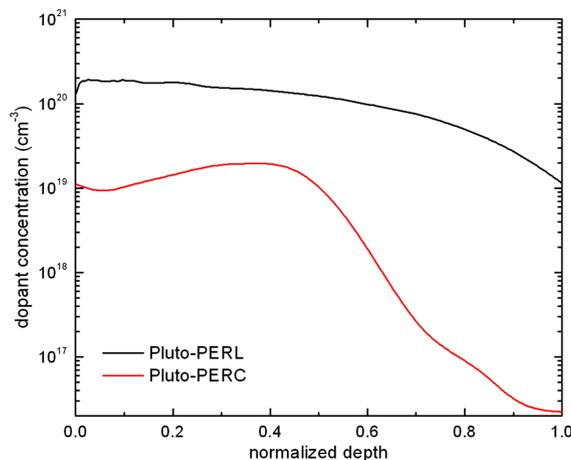
**Figure 5.** Electrochemical capacitance voltage doping profile of the rear p-type silicon opening for Pluto-passivated emitter and rear cell (PERC) and passivated emitter and rear locally diffused (PERL) cells. The depths of the  $p^+$  regions are normalised to that of Pluto-PERC.
