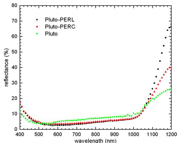
**Figure 4.** Corresponding reflectance curves of the next-generation Pluto cells in Figure 3. Reflectance data for conventional Pluto cells were extracted from Ref. 8 and included for comparison.
