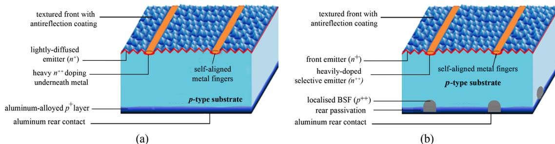
**Figure 1.** Schematic of (a) the first-generation Pluto cell with rear surface covered entirely with aluminium corresponding to 100% contact area for the metal/silicon interface surface [8] and (b) the next-generation Pluto cell with localised rear contacts.
