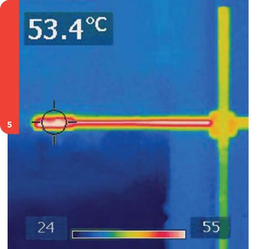
Effective temperature control is essential to prevent early life failure as it is proven that excessive temperature reduces the performance of LEDs leading to a shorter life span, reduced efficiency and disturbance in colour. The cooler the LED, the longer the life
