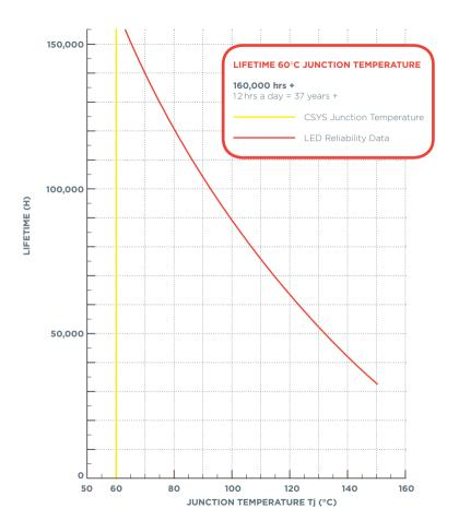
Please refer to the graph on the opposite page which outlines the projected life of the LED chips within the CSYS task light. These figures are achieved thanks to the refined and efficient heat management of the heat sink within the CSYS task light.
