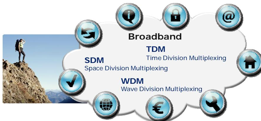
The SDM approach is based on keeping the bit rate the same but use more fibers – durable for short geographical distances and it is the most straightforward upgrade alternative. However it has two main drawbacks. It requires more fibers and for long geographical distance optical amplifiers for each fiber set – driving the cost up.
