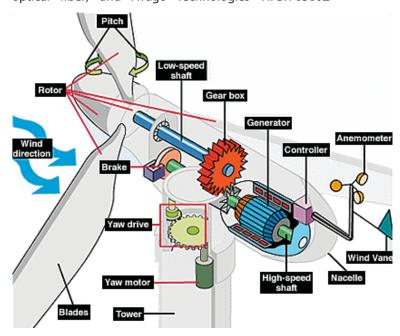
Figure 4. Elements within a Wind Turbine Nacelle Requiring Fiber Communications
