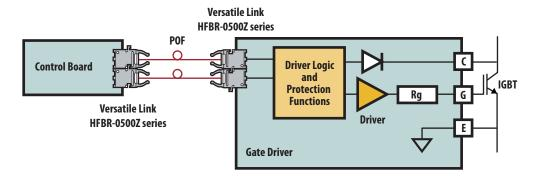
Figure 2. IGBT Gate Driver Block Diagram
