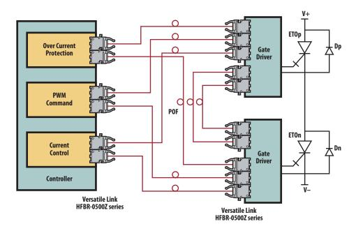
Figure 3. ETO Two-Level Voltage Source Converter Phase Leg Block Diagram
