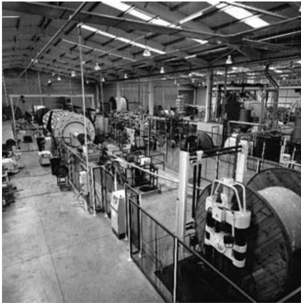
Figure C6.36 Twin carriage armouring machine [photograph courtesy of JDR Cables]
