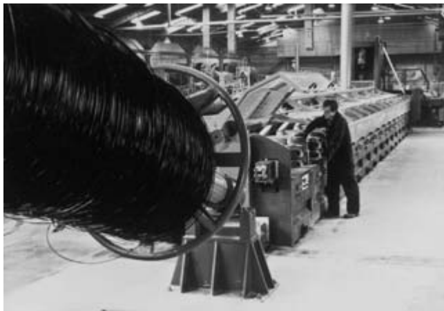
Figure C6.35 Wire drawing machine [photograph courtesy of Bridon International]
