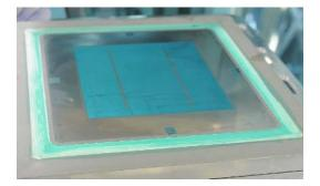
Figure 2: The print screen contains a pattern of open and closed spaces that allow paste to wafer transfer.
