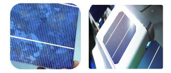
Figure 4: The frontside of the wafer after printing shows large and small contact lines that collect electricity from the active regions.
