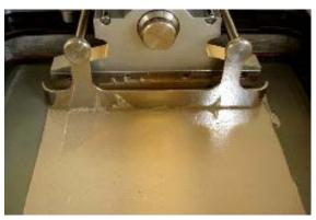
Figure 3: After conductive paste is dispensed onto the screen, the squeegee spreads it across the screen and presses it through onto the wafer.
