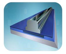
*Figure 9: Double printing over selective emitter*
