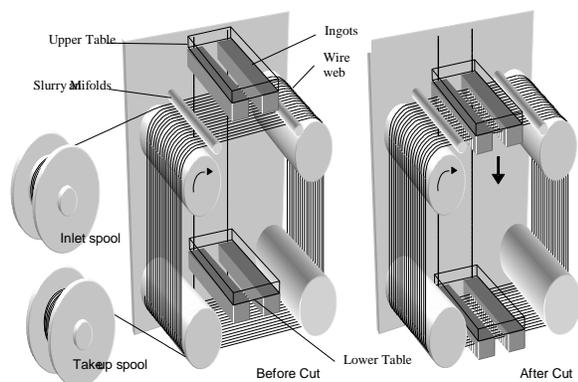
Figure 3: Schematic of a multi-wire saw. Silicon blocks are passed through the web of cutting wires.
