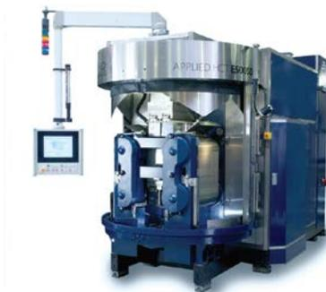
Figure 4: The Applied HCT B5 Wire Saw
